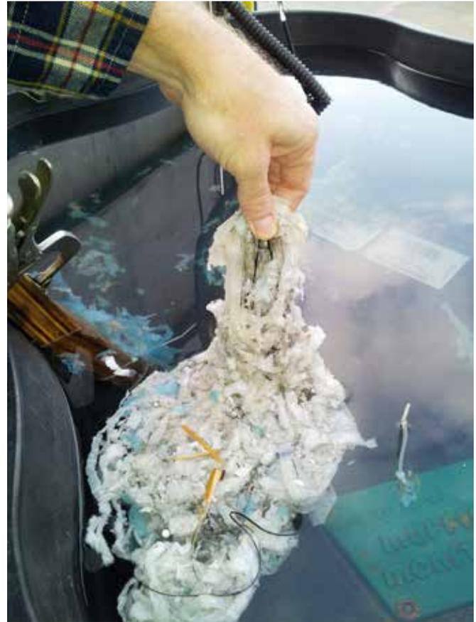
**Rag balls form in collections systems when debris and hair knit together. Research revealed that hair is the main catalyst for the rag balls.**
